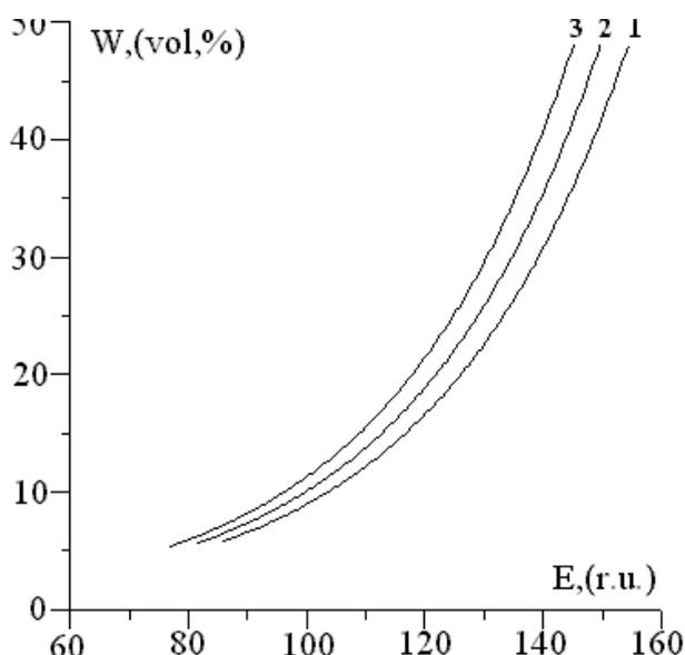
Fig.1 Water content in vol% as a function of the scatterometer intensity  $E$  calculated using a priori data on the soil texture of the Chernobyl area. (1) is sandy (2) sandy loam and (3) is loamy soil.
