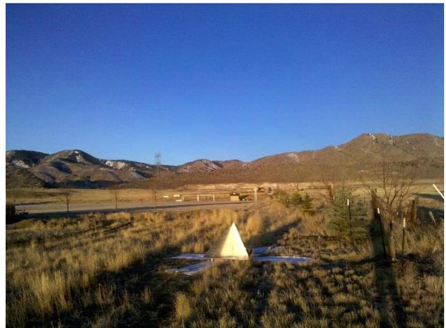
Figure 11. Large reflector (1 m by 1 m by 1.4 m)
