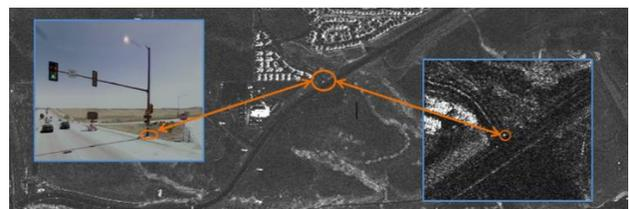
Figure 2. Location of a metal pole in the SAR data
